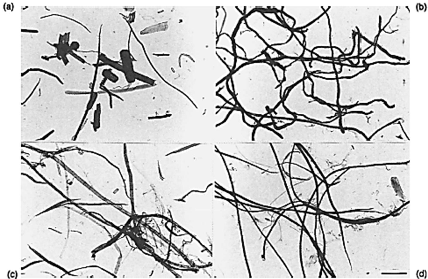
**Figure 1.2** Light photomicrograph illustrating morphological differences between cell and fibre types of non-woody pulps: (a) straw (stem residue), (b) cotton (seed hair), (c) flax (stem), (d) Abaca-Manilla hemp (leaf fibre). All fibre preparations have been stained for clarity. Scale bar = 200  $\mu\text{m}$ .
